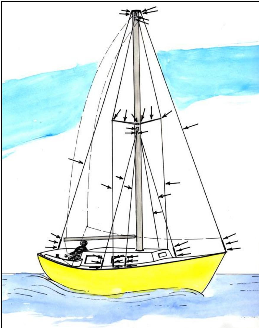
*Lose any one part of a piece of standing rigging, and the whole rig can come crashing down. Many of the parts are up high and out of sight, so even detecting the onset of a failure is problematical because inspection requires a fair amount work, and so is done rarely.*
