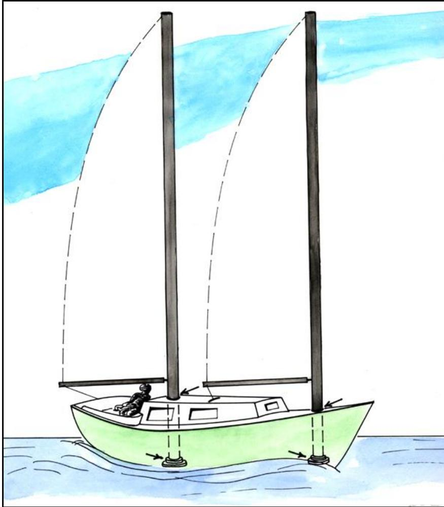
*Free-standing masts are held by two parts, the heel fitting and the deck fitting. These are substantial structures that are close at hand for easy inspection. Failure here is very unlikely, and the onset of failure is easily detected because the parts are easily inspected.*
