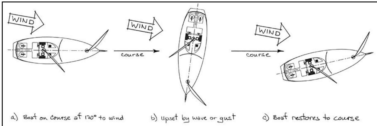
A free-standing wingmasted boat like *Project Amazon*, pictured here, can sail fast deep downwind with the booms set forward of abeam wing-and-wing (a), something which no other boat with a stayed rig can do. If a gust or wave upsets the boat, even to turn it broadside to the wind (b), the sails will pull the boat back on course (c). This makes the boat naturally stable and almost totally immune to crashing gybes and broaches.
