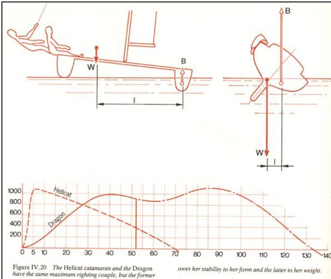
Pierre Gutelle, *The Design of Sailing Yachts*, International Marine Publishing, first edition, 1979. This shows a typical comparison between the righting curves of a small multihull and small monohull. Note that the peak of the multihull curve occurs at a small angle of heel, whereas the peak of the monohull curve occurs at a much larger angle of heel. The multihull will see its maximum load much more frequently than a monohull will. This has to be taken into account when designing the mast.
