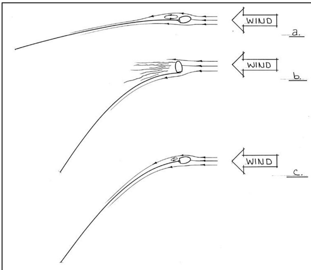
*When sailing on the wind (a), the airflow on the back side of the mast is well-attached. Off the wind (b), the flow separates easily on the back side of a non-rotating mast, producing almost pure drag. By allowing the mast to rotate into the wind (c) the airflow remains attached and generates considerable lift.*
