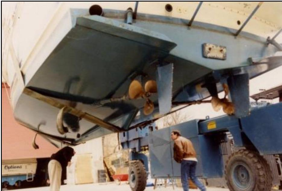
**Fig. 6.** When we lifted the 34' sedan cruiser in the Travelift, we found the bent propeller.
