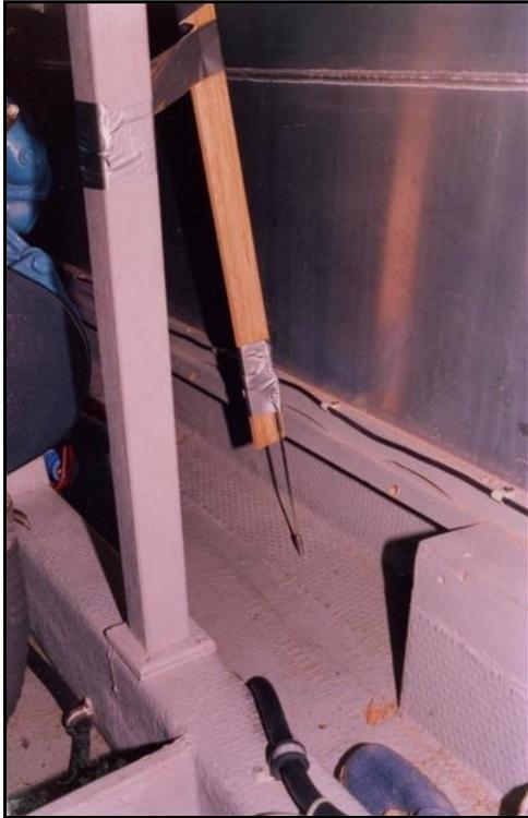
**Fig. 4.** *The telescoping wand touching on an outboard hull panel gave us an indication of how much the bottom moved.*
