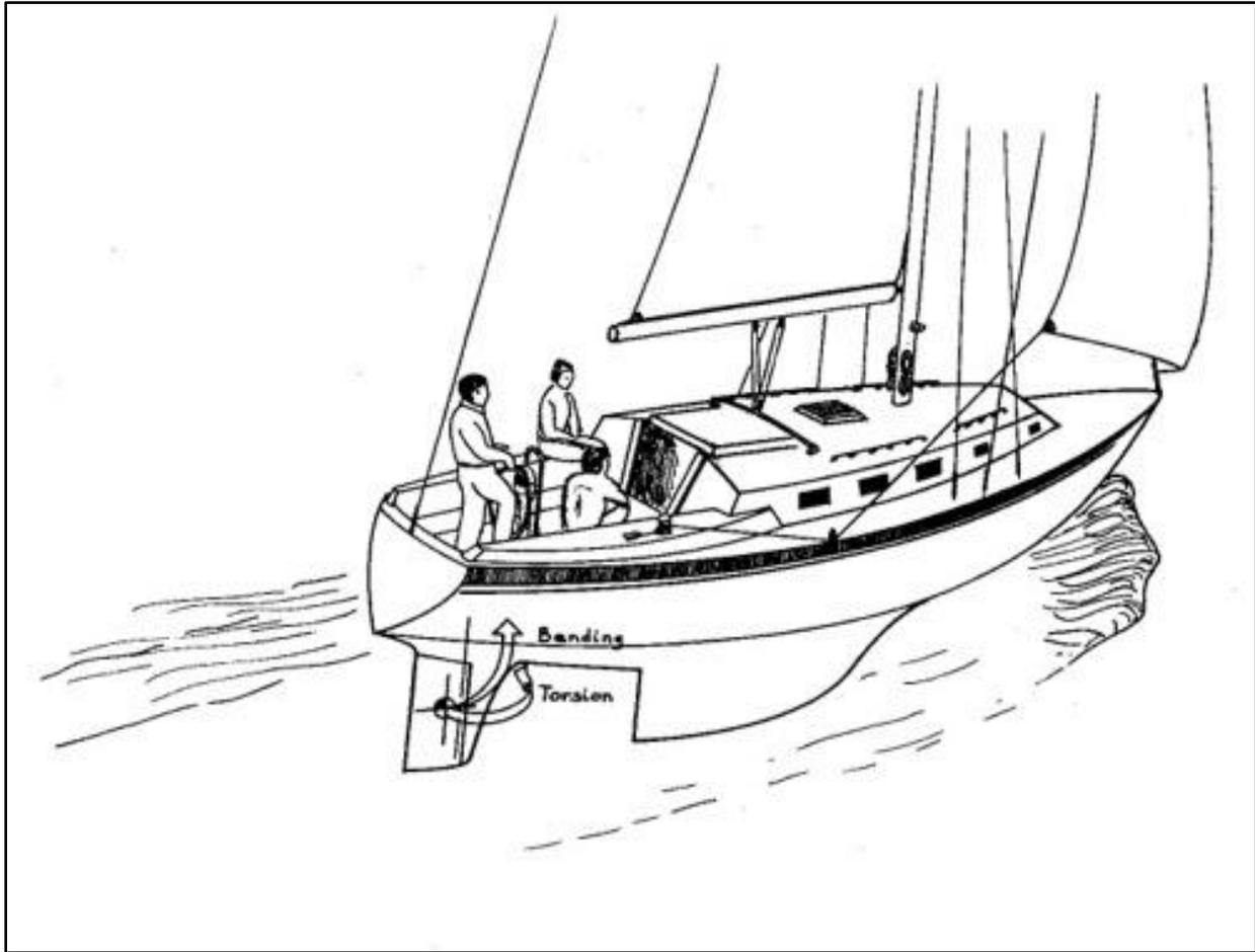
*Fig. 6. The bending and torsion loads on a rudder.*
