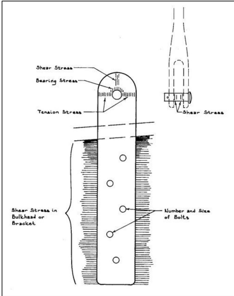
*Fig. 7. These are the areas to engineer in a chainplate.*
