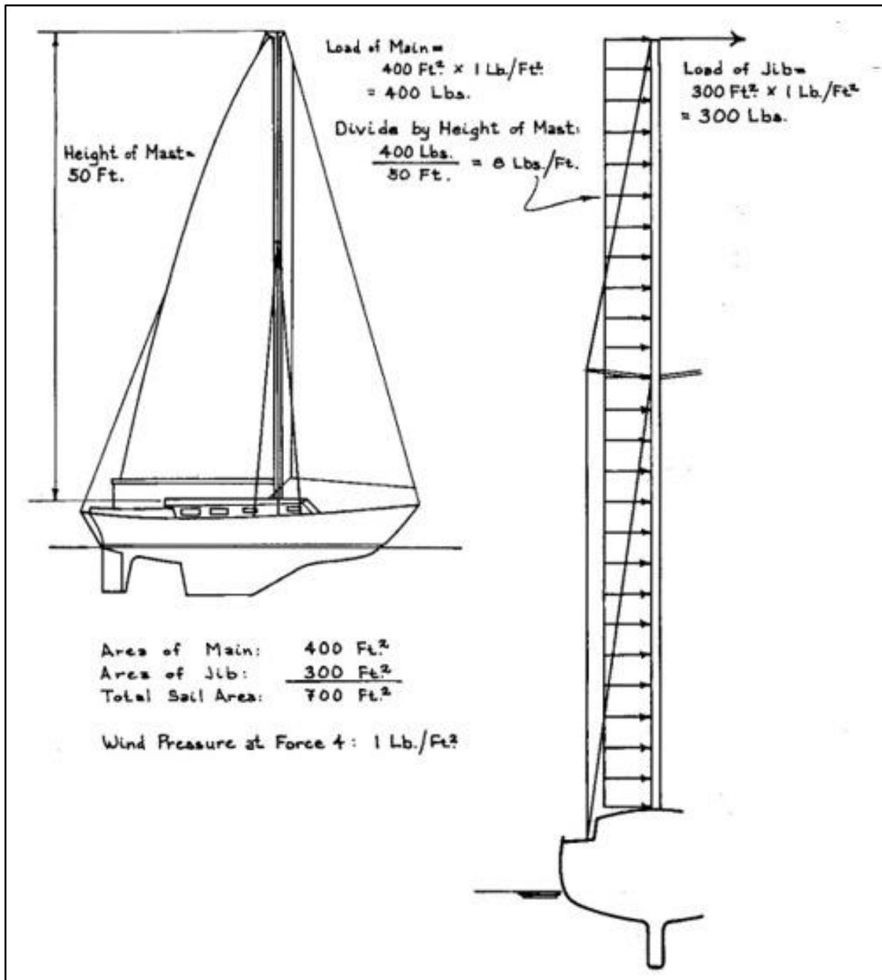
**Fig. 1.** The basic loading on a mast.
