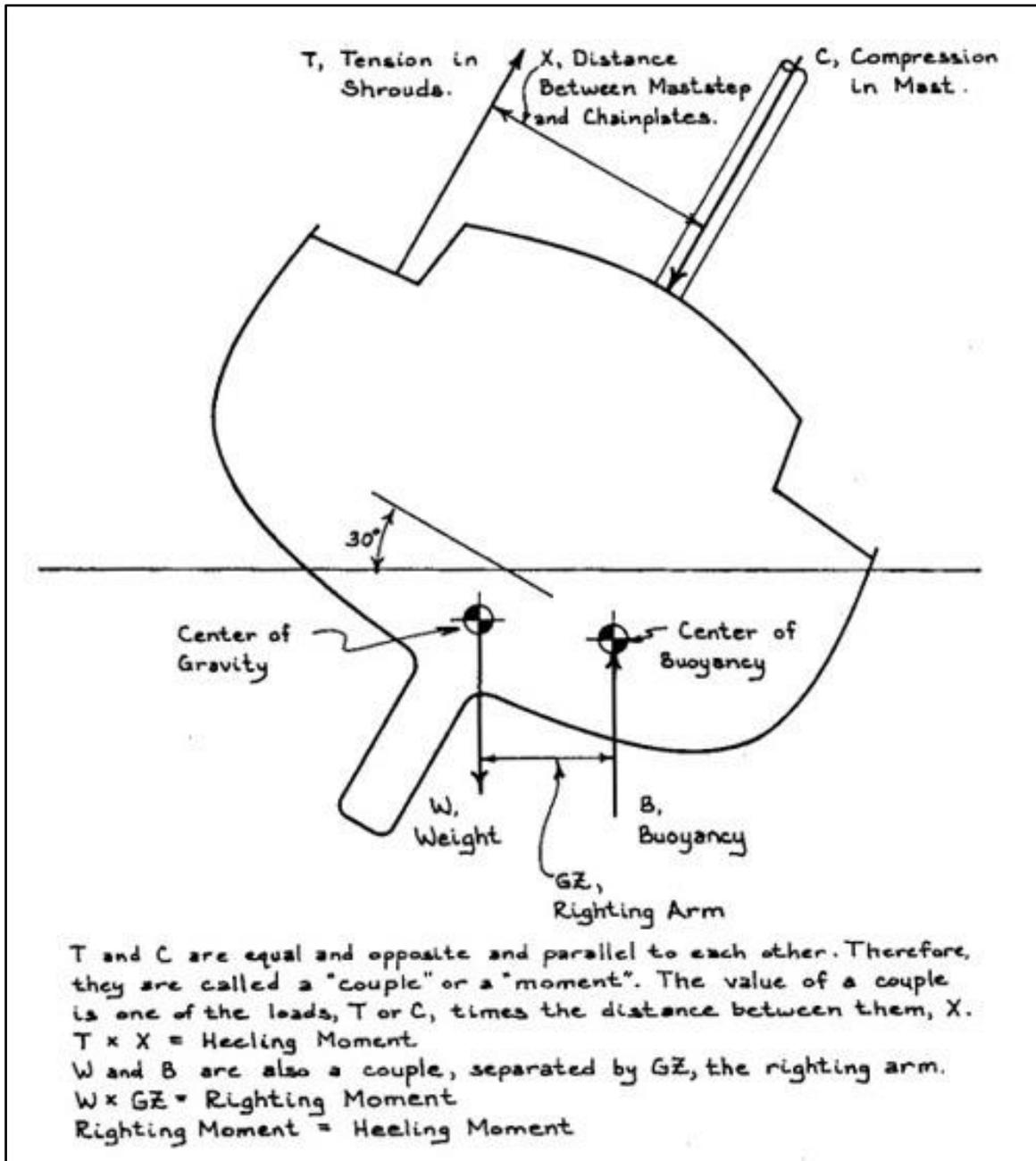
**Fig. 2.** Mast compression and shroud tension form a couple that is equal to the couple created between the boat's weight and buoyancy. In fact, to engineer a sailboat rig, you can ignore the heeling moment created by the loading by the wind on the sails and start with the boat's righting moment. By definition, righting moment and heeling moment are equal and opposite.
