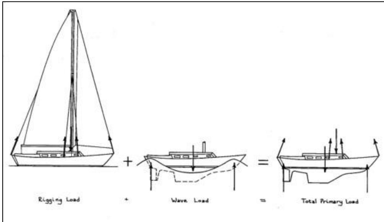
**Fig. 3.** Primary loading on the hull of the combined rigging and wave loads
