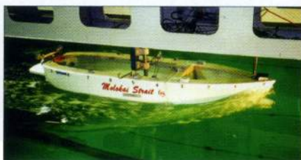
Left —Hercules, finished out by St. Augustine (Florida) Marine, is shown here in primer. Note the nabla-style bulbous bow. Above —Model testing at Oceanic Consulting and the Institute for Marine Dynamics, in Newfoundland, was one of the most worthwhile and important exercises in the design process. It clearly defined the resistance characteristics of the Moloka'i Strait hullform, which translated directly to the MS 75 Hercules.
