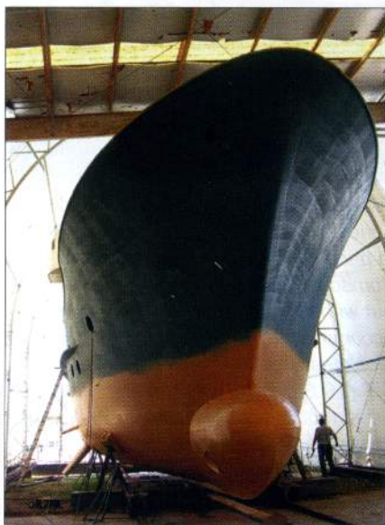
Left —Hercules, finished out by St. Augustine (Florida) Marine, is shown here in primer. Note the nabla-style bulbous bow. Above —Model testing at Oceanic Consulting and the Institute for Marine Dynamics, in Newfoundland, was one of the most worthwhile and important exercises in the design process. It clearly defined the resistance characteristics of the Moloka'i Strait hullform, which translated directly to the MS 75 Hercules.
